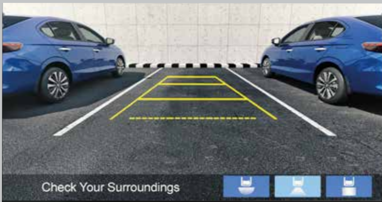
MULTI-ANGLE REAR CAMERA WITH GUIDELINES (NORMAL, WIDE, TOP-DOWN MODES)
